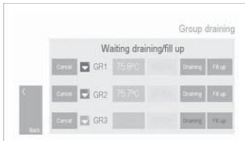
Press the 'Emptying' button and then the group or groups will start emptying through the purge hole of the solenoid valve and the air purge.
