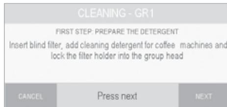
Once you have added the detergent to the blind filter and affixed the filter holder in the group, press 'Next' to go to Instruction No. 2 which tells you to press the central key of the group to be flushed, which will be flashing, to start the process.
