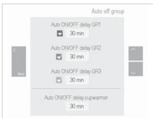
To activate the group again, simply press any button of the deactivated group and it will start heating up again until it reaches the pre-set service temperature.
