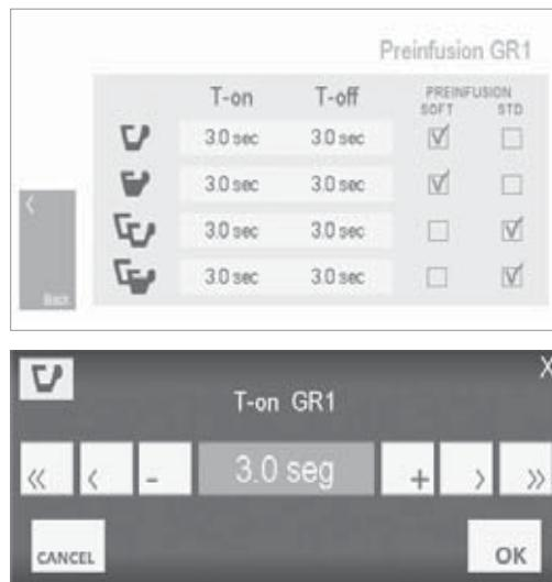
In both cases, there is an 'on' time during which the water moistens the coffee, and an 'off' time when the ground coffee tablet is soaked completely before the distribution starts at 9 bar.
