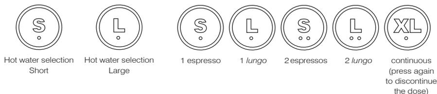
To program the amount of coffee (volumetric dose) or hot water (set by time, not volume), with the machine ON and ready to make coffee (keys of the keypad permanently lit), press the programming button XL for 5 or 6 seconds until it is lit intermittently while the rest of the keys are illuminated in a fixed manner.
